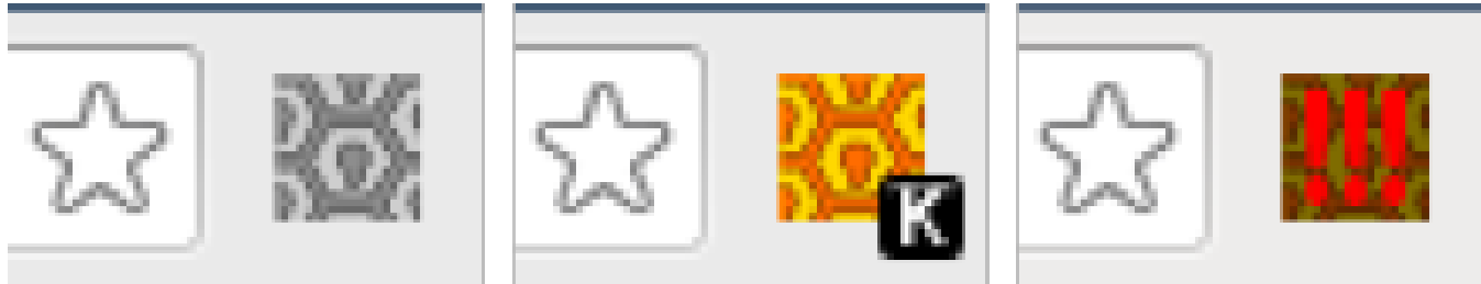
Fig. 2. The Privacy Indicator “unprotected” (left), “protected” due to keyboard events (“K”) in a private area (middle), and showing a security warning (right).
