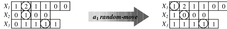
Fig. 7. The violation numbers are updated, when agent a_1 moves to a new position by executing a random-move behavior.
