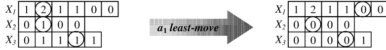
Fig. 5. The violation numbers are updated, when agent a_1 moves to a new position by executing a least-move behavior.
