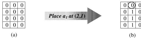
Fig. 28. (a) Violation numbers at the initialization step. (b) Violation numbers updated having placed a_1 at (2,1).
