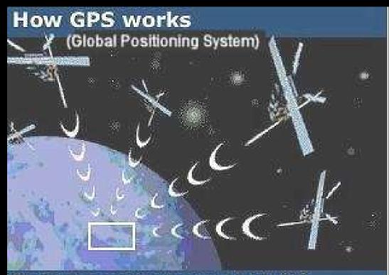
The Earth is continually circled by 24 GPS satellites. At least four are always visible from any one point. Your GPS receiver listens for signals which give the satellites' location and the exact time of sending. Triangulation then gives your latitude and longitude to within 100m.
