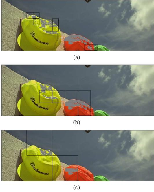
**Fig. 2:** Illustration of the level-based block extraction employed in the hierarchical windowing algorithm corresponding to (a) 32x32, (b) 64x64, and (c) 128x128 block sizes. The gray shaded areas indicate the saturated regions at each level.
