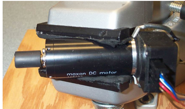
Figure 1: Haptic display. A brass knob mounted directly on the motor shaft was covered with stiff rubber to prevent slipping. The vise mounting allowed adjustment of motor position for each participant.
