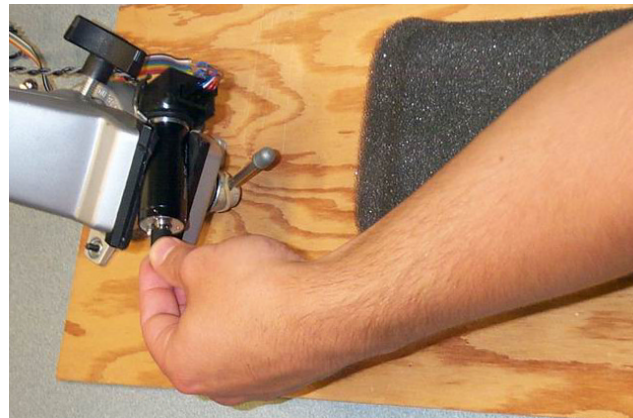
Figure 2: Setup. Participants were asked to hold the knob lightly between their thumb and index finger as shown here. The haptic knob was placed horizontally in a position easily reachable by the participant while resting the forearm on a cushioned armrest.
