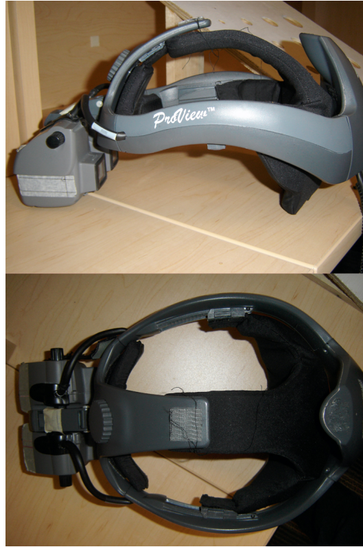
Figure 3.3: The Kaiser ProView XL50 head mounted display. The vertical line on the tape attached to the left optical module indicates the position of the z-position of view screen used.
