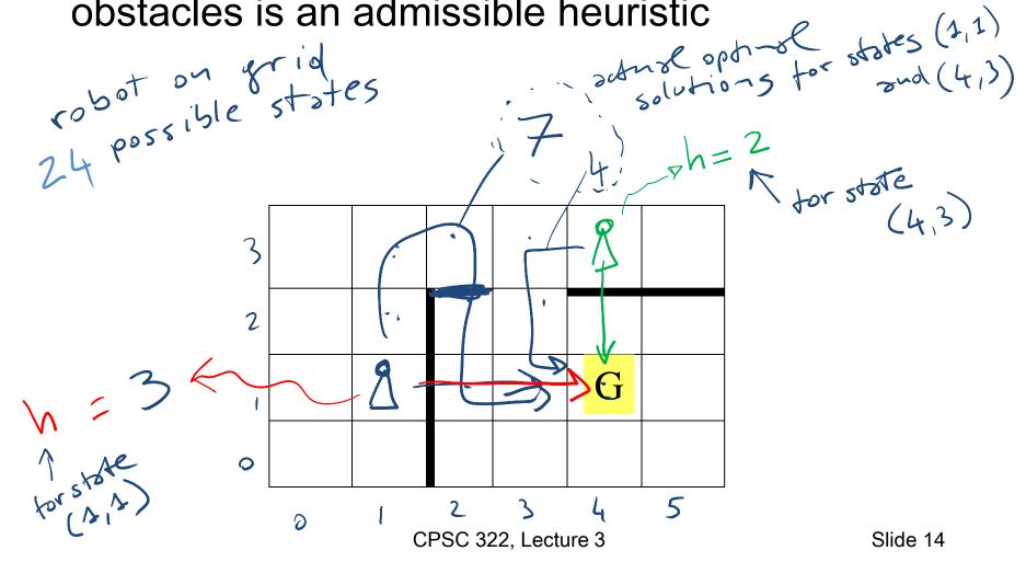
Similarly, If the nodes are points on a Euclidean plane and • the cost is the distance, we can use the straight-line distance from *n* to the closest goal as the value of h(n).
