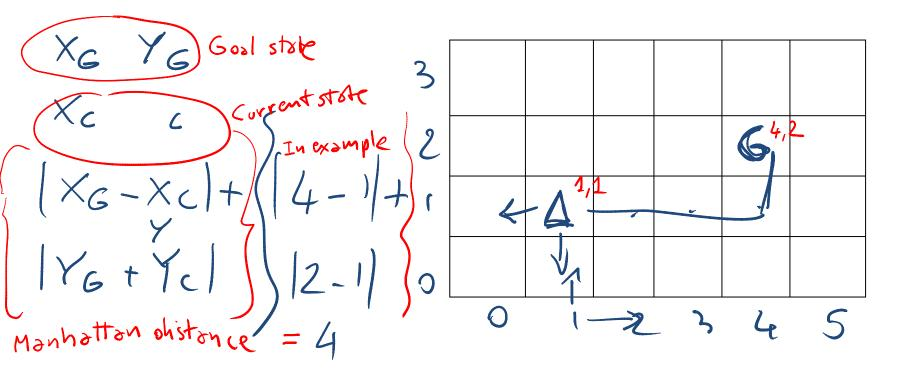
If there are obstacle, the optimal solution without obstacles is an admissible heuristic
