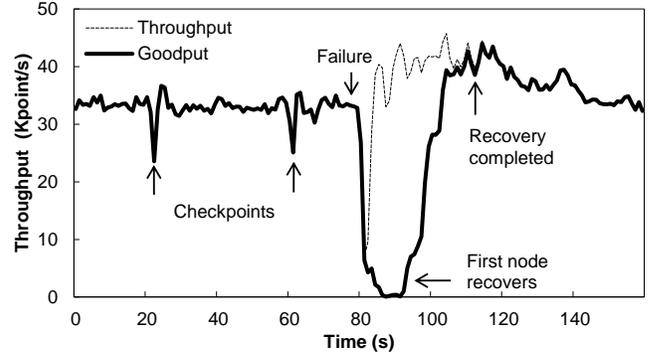
Figure 11. Throughput and goodput over time as Sonora checkpoints twice and then recovers from a failure.
