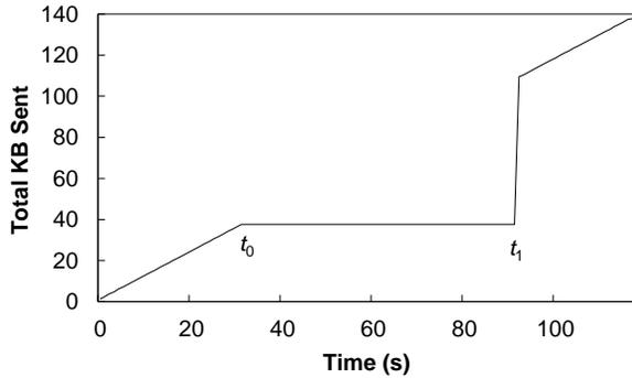
**Figure 12. Total KB sent over time with a sync stream. A disconnection is masked between  $t_0$  and  $t_1$ .**
