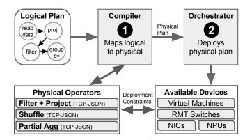
Figure 2: Overview of the how Jumpgate will interact with a data processing system to compile and orchestrate in-network processing.
