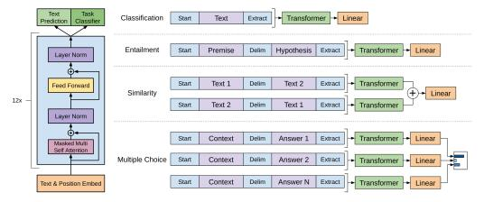
Figure 1: (**left**) Transformer architecture and training objectives used in this work. (**right**) Input transformations for fine-tuning on different tasks. We convert all structured inputs into token sequences to be processed by our pre-trained model, followed by a linear+softmax layer.
