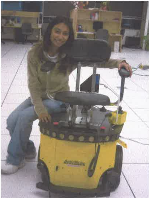
Figure 11. Prototype Smart Wheelchair (UBC, 2006)
