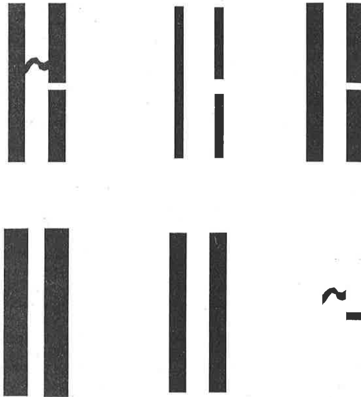
Figure B-11. Application of opening and closing to PC board inspection.
