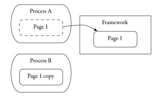
Figure B.5: After modifying a read-only virtual memory page. The page is copied to the the address space of the patching process.
