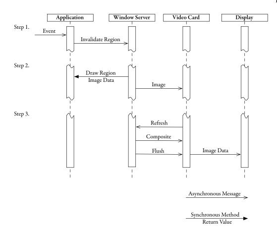
Figure 2.9: Sequence of events causing an image to be drawn to a display device.
