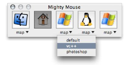
Figure 2.12: The Mighty Mouse (Rover) toolbar. This toolbar is used to move the cursor between PCs in the system. The dropdown menu shows the cross-platform keyboard translation mapping in use on the machine being controlled.
