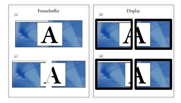
Figure 3.2: Effect of a positive screen gap on image display. For the upper image, a standard extended desktop is used that has two abutting screens in the framebuffer (a), and the physical dimensions of the image have been stretched when viewed on the two displays (b). By logically separating screens in the framebuffer (c), the bezels between displays can be compensated for, maintaining the aspect ratio of GUI objects spanning the displays (d).
