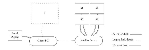
Figure 4.3: Logical display consolidation. In this example, a graphics cluster acts as a satellite display, tiling 4 displays (S1-S4) into one device that is presented to the client PC as one large logical display (S).
