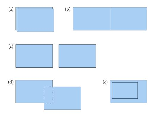
Figure 1.1: Possible relationships between two screens in two dimensions. The familiar mirrored mode is shown in (a), while the arrangement in (b) indicates extended desktop mode. There is a logical gap between screens in (c), and the screens in (d) and (e) have varying degrees of overlap.
