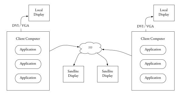
Figure 4.2: Proposed system overview. Each client computer is connected to a local display via a traditional DVI or VGA link. They are also simultaneously connected to multiple satellite displays through a mechanism that is left unspecified in this idealized view.
