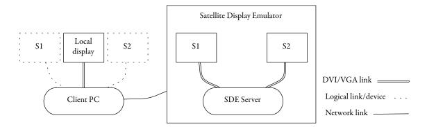
Figure 5.3: Individual display export. In this case, each display (S1, S2, solid outline) attached to the SDE Server is exported individually. The satellite displays may then be positioned independently on the client PC. This allows a user to create the arrangement shown at left, where a local display is inserted between two satellite displays (S1, S2, dashed outline).
