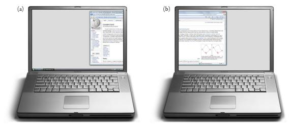
Figure 2.7: Maxivista. The user's computer (a) has a *secondary display* attached through the use of a special graphics card driver; anything that is rendered to the proxy secondary display is captured, sent over a network, and displayed on a different computer (b).
