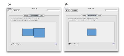
Figure 3.1: Configuring multiple displays on Mac OS x. Iconic representations of extended desktop (a) and mirror mode (b) are shown.
