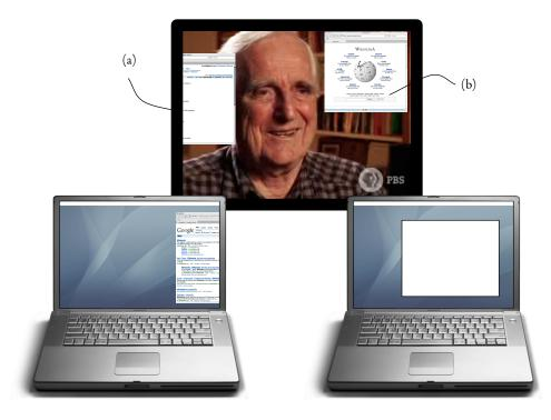
Figure 4.7: Sharing content on a home entertainment display. In this example, the laptop on the left has a window partially shared onto the TV (a), and the laptop on the right has a fully shared window (b).
