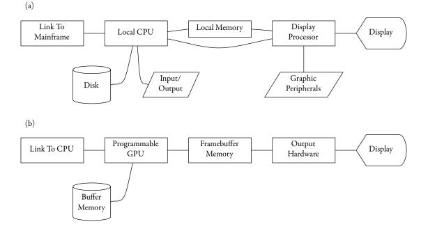
Figure 4.1: Graphics system block diagram. Mainframe / satellite system circa 1974 (a), GPU circa 2006 (b).
