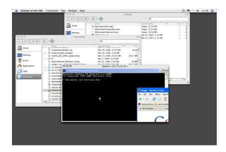
Figure 2.11: Single window sharing with UltraVNC. Note that the *single window* includes a portion of an Internet Explorer window, due to the way the Windows XP window server composites directly to the framebuffer.
