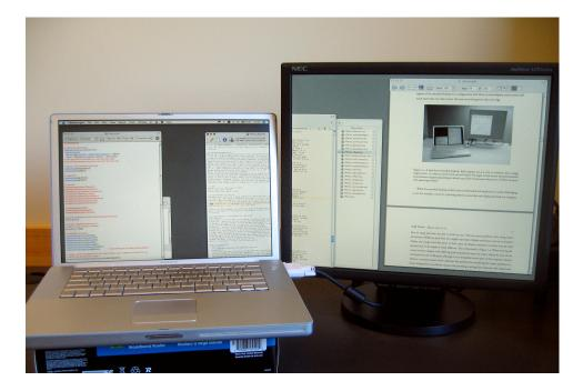
Figure 2.3: A dual-head extended desktop. Both displays act as a view or window onto a larger virtual screen space; GUI objects can be freely moved within this larger virtual screen and automatically move between displays depending on which area of the virtual screen they are in. In this example, one GUI window straddles the two displays, with different portions shown on each.
