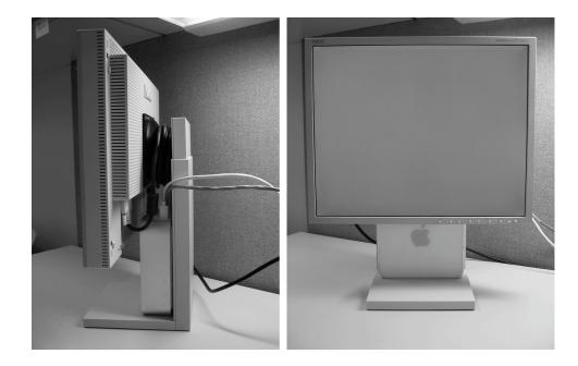
Figure 5.1: Prototype satellite display. The Mac Mini computer used to prototype the graphics and networking functionality is small enough to fit within the frame of the LCD panel. There are three cables used to connect the prototype satellite display: power for the display, power for the PC, and Cat-5 networking.
