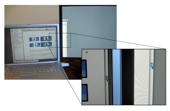
Figure 3.6: Extended desktop with partial overlap. In this example, the scrollbar exists on both displays, allowing the user to easily acquire it from either the left or the right.
