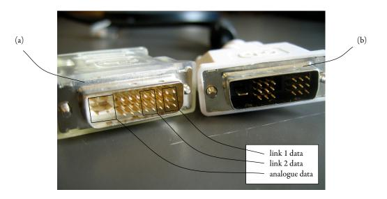
Figure C.1: Different DVI connectors. In a DVI-I (dual-link) connector (a), both analogue and digital signals are supported. In a DVI-D connector (b), the connector is missing the four analogue pins surrounding the large flat pin, and the central six pins for the second digital link.
