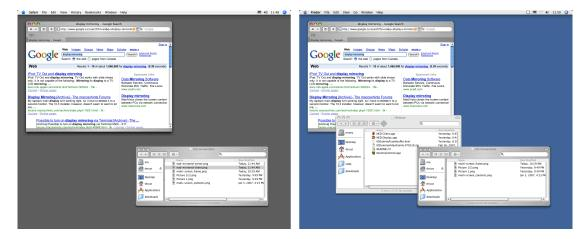
Figure 5.9: An SDE compositing multiple sources. A user's display (a) is mirrored on an SDE display (b). In addition, a second user has placed an additional window on the SDE display. Note how it has been inserted between the two windows from (a), overlapping one and being overlapped by the other.
