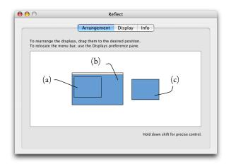
Figure 3.3: The Reflect configuration window. This view behaves similarly to the built-in Display Arrangement preference panel, but allows display proxies to be dragged anywhere in screen space. In this example, three displays have been configured, one properly inset (a) in the main display (b), and one disjoint off to the right (c).
