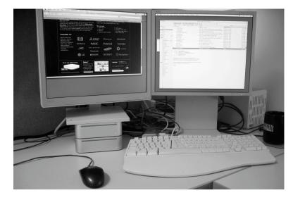
Figure 2.8: Multiple computers sharing one keyboard and mouse. In this figure, both hardware (a KVM) and software (the synergy input redirection tool) are used to transfer input events between computers, depending on the task.
