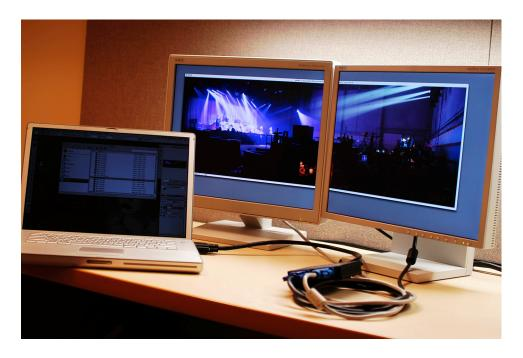
Figure 2.6: Matrox DualHead2Go. This device accepts a video signal at display resolutions twice as wide as a normal display, and logically splits the image for output to two display devices, each having normal width.
