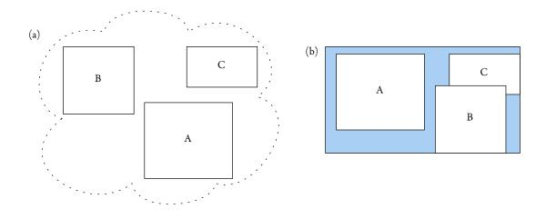
Figure 4.5: Fine-grained GUI object transmission. The GUI objects that make up a screen may be sent individually (a), and all of the compositing is done on the satellite display (b).
