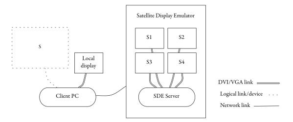
Figure 5.4: Tiled display export. In this example, the SDE pre-tiles four displays (S1-S4), and exports them as a single large display (S) to the client PC.
