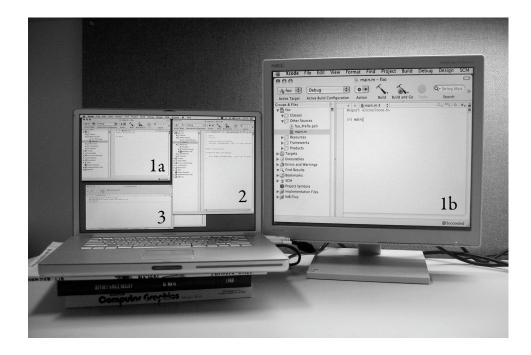
Figure 3.4: Inset mirroring example. The external display (1b) only shows the top left corner (1a) of the laptop's built-in display. This allows a portion of the screen to be mirrored, while omitting unnecessary clutter.
