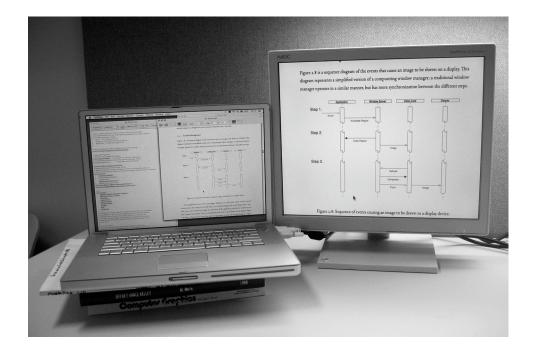
Figure 3.5: Inset mirroring used as a magnifier. The external display shows a zoomed in subregion of the laptop's built-in display.
