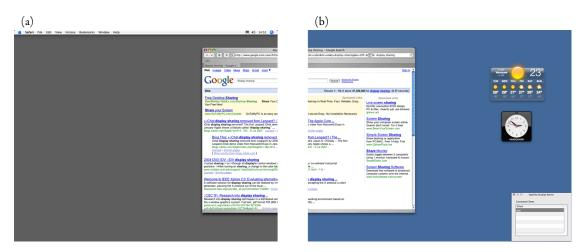
Figure 5.7: An SDE with local content. The local display is on the left (a), and the output from the SDE on the right (b). In this example, the SDE locally hosts a weather and clock widget, which remain on-screen regardless of whether a client PC is connected or not. In addition, a diagnostic window for the SDE Server software is shown at the bottom right; this lists the currently connected client PCs.
