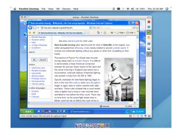
Figure 2.10: Virtualization Environments. Microsoft Windows running on a Mac OS x computer, within the Parallels virtualization environment.
