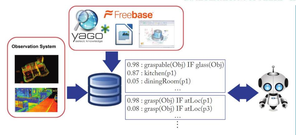
**Figure 1.7:** The robot's relational probabilistic model is populated with the data produced by its perception and experience (robot log data, human motion tracking, environment information, etc.) as well as with facts (or assertions) extracted from other dark data.
