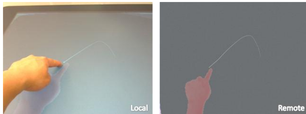
Figure 2. Arm shadows are displayed locally as feedback, as well as at remote sites. Finger contacts are transmitted to remote sites, and conveyed via trace pearls: the contact point is represented by a small disc, and the trail fades over time.
