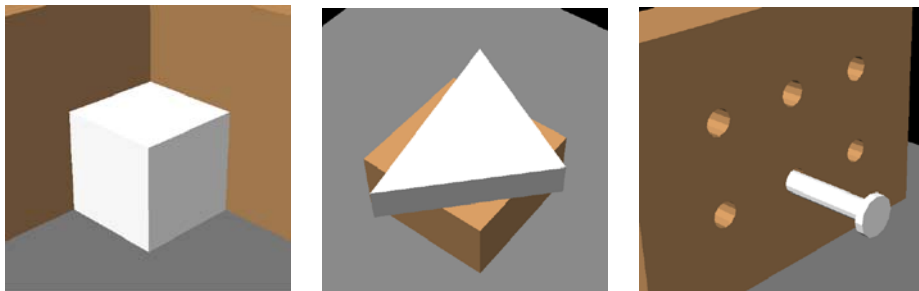
Figure 1: Some extended contacts with numerous contacts points. Left to right: block-in-corner (12 contacts), face-on-face (6 contacts), peg-in-hole (arbitrary contacts).
