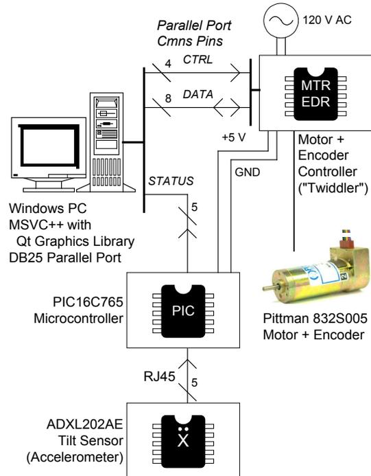
Figure 4: I/O controller components
