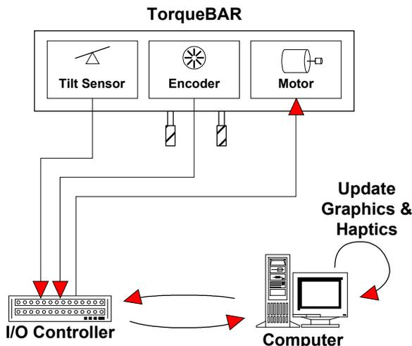
Figure 3: High-level data flow
