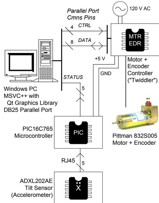
Figure 4: I/O controller components
