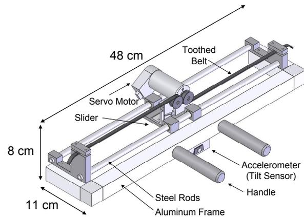
**Figure 2: TorqueBAR physical interface. The device’s centre-of-mass moves when the motor turns, pulling the motor along the device’s rails**
