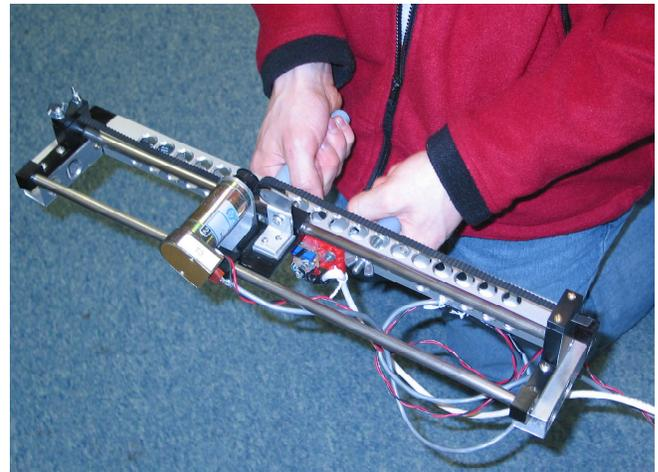
Figure 1: TorqueBAR ungrounded force feedback device
