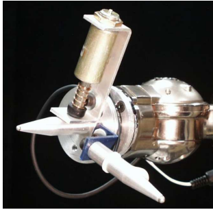
Fig. 4. Tri-headed sensing tool, including (clockwise from top) solenoid-driven sound effector (for acoustic impulse response), contact-microphone probe (for scraping sounds), and a friction/roughness probe. The force sensor is located directly behind the sensing tool
