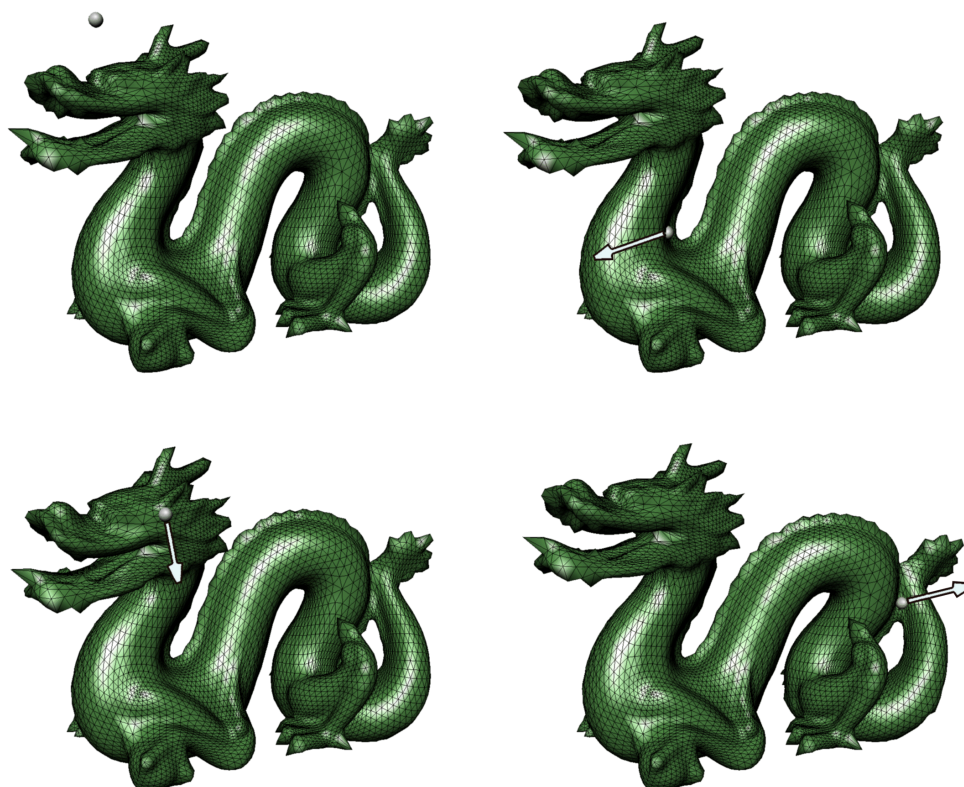
Fig. 22. Deformed dragon model ( L = 3 ) shown in a force feedback simulation, contacted by a small white ball (force direction indicated by arrow). The undeformed model is shown in the top left image, while other images illustrate hierarchical GF deformations due to forces resolved on constraint level 0. This very large model compresses extremely well (approx. factor of 100 at 5% RMS error) and is therefore suitable for interactive force feedback simulation.
