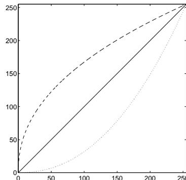
Figure 1: Gamma correction as a function of intensity. (solid)  $\gamma = 1$ ; (dashed)  $\gamma = 0.45$ ; (dotted)  $\gamma = 2.22$ . Note how, for  $\gamma < 1$ , the lower intensities are mapped onto a larger range.
