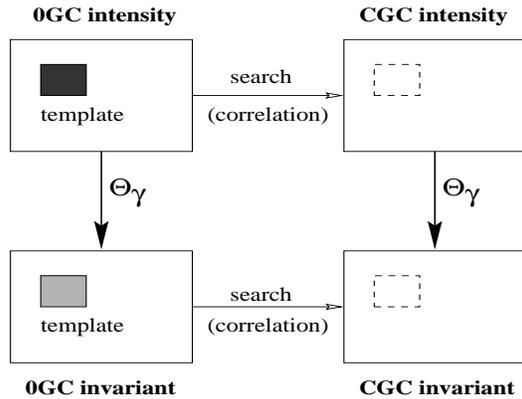
Figure 7: The template location problem: A query template is cut out from the OGC intensity image and correlated with the corresponding CGC intensity image. We test if the correlation maximum occurs at exactly the same location as in the OGC intensity image. The same process is repeated with the invariant representations of the OGC and CGC images.
