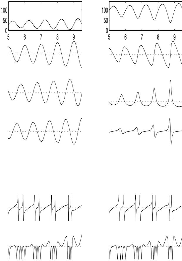
Figure 2: An analytical example function. (left)  $f(x) = 3x \sin(2\pi x) + 30$ ; (right)  $f_\gamma(x) = p f(x)^\gamma$ ,  $\gamma = 0.45$ . (first row) original functions (second row) first derivatives; (third row) second derivatives; (fourth row) third derivatives; (fifth row)  $\Theta_{m12\gamma}$ ; (sixth row)  $\Theta_{m123\gamma}$ .
