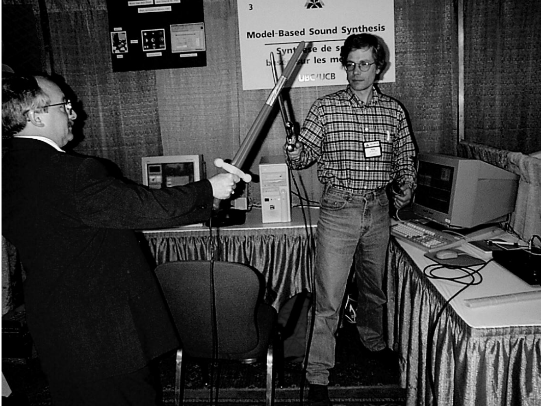
Figure 7.6: Plastic swords with embedded contact mikes used to create metal sword sounds.
