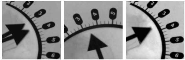
Figure 6. Subframe warping synchronization. Left: two consecutive overlaid fields from first camera. Center: closest integer frame aligned field from second camera. Right: warped field from first camera, synchronized to match the second.
