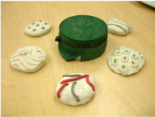
Figure 1: The variable-texture surface prototype. A latex membrane (center) is stretched over a section of tube. Clay surfaces push against the membrane underside to alter its texture.
