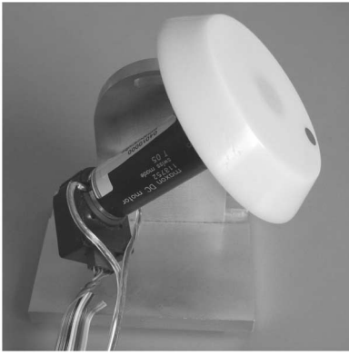
Fig. 5. The haptic interface knob, motor, encoder, and stand.
