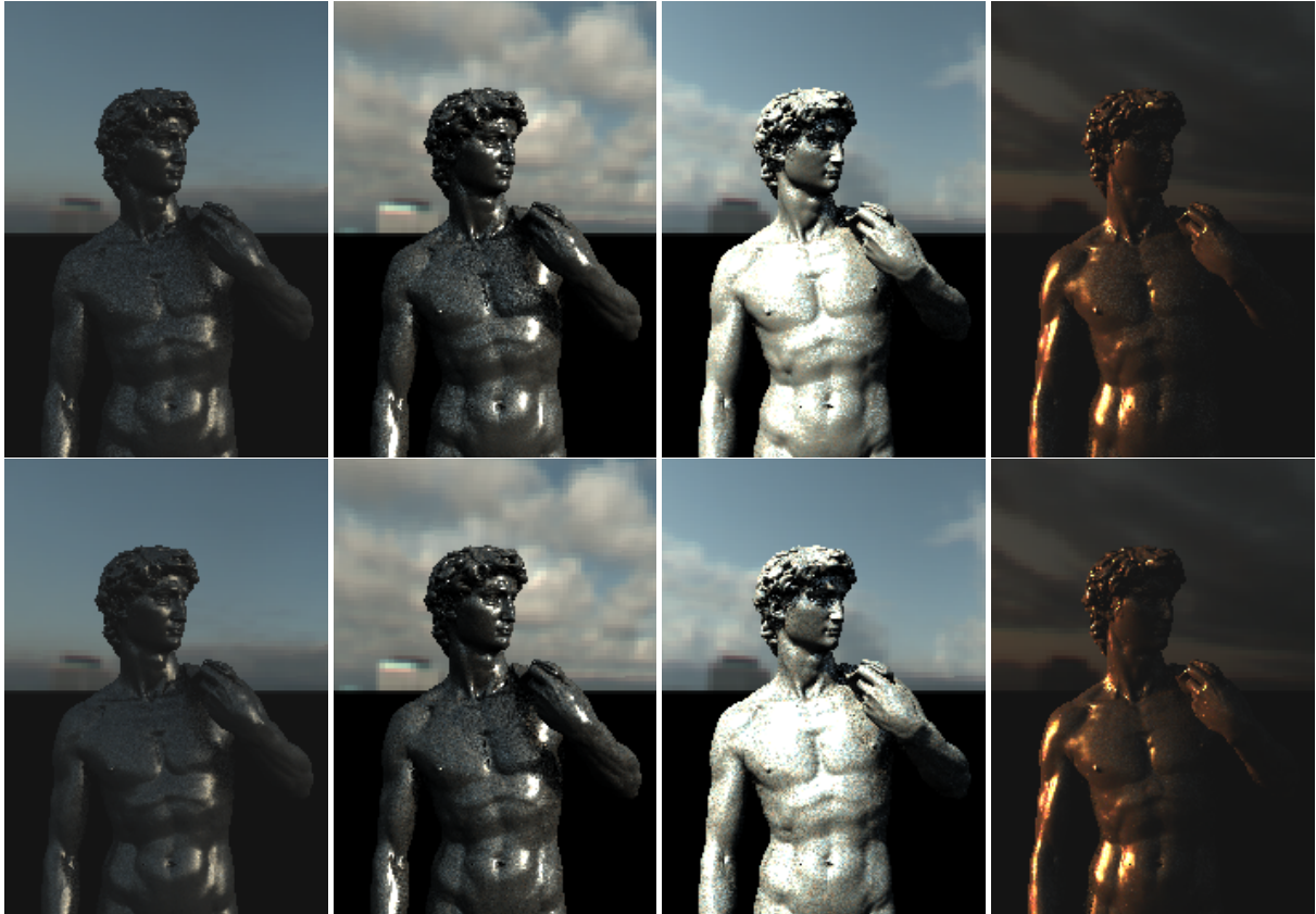
Figure 5: Quality comparison between bidirectional sampling and our SMC sampling algorithm for a BRDF with a diffuse component in the sky probe gallery sequence. Top row: Bidirectional sampling ( N = 16 , M = 200 ). Bottom row: SMC sampling ( N = 16 , P = 5 , path sampling). All images took the same compute time of 4 seconds.
