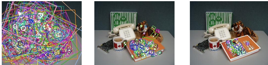
Figure 4: Finding consistent sets of feature matches. To find inliers to a homography we use a Hough transform followed by RANSAC. In this example, the test image was 640 \times 512 pixels. The number of initial matches to consider was 5469, which was reduced to 279 by broad-bin Hough transform clustering, and further to 104 matches in the final solution using RANSAC.
