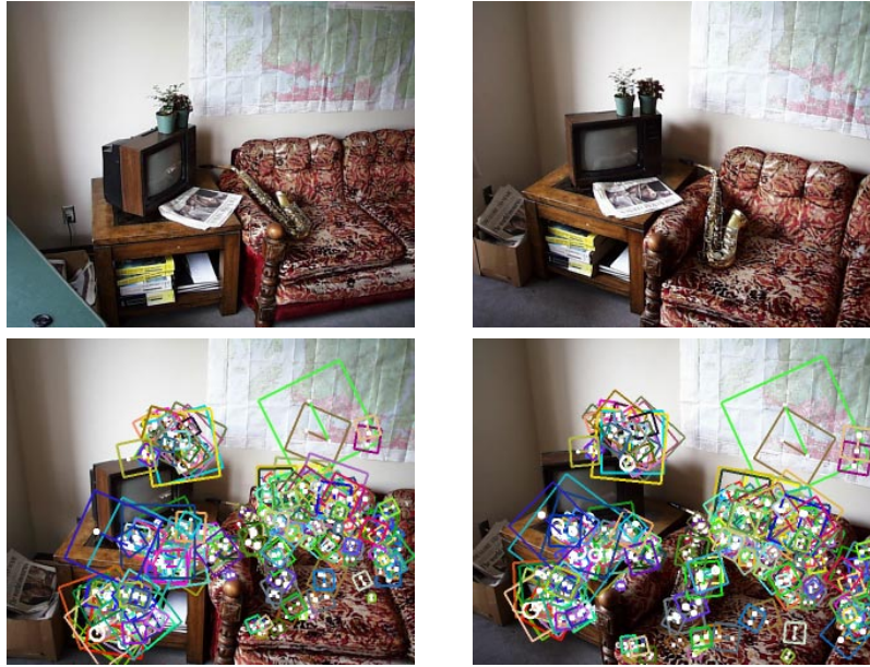
Figure 1: Matching of invariant features between images with a large change in viewpoint. Each matched feature has been rendered in a different greyscale.
