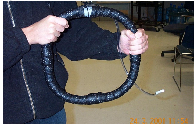
Figure 5. Haptic steering wheel. Built from PVC conduit and a vinyl steering wheel cover; the pneumatic display is located beneath the steering wheel cover, under the subject's right hand.
