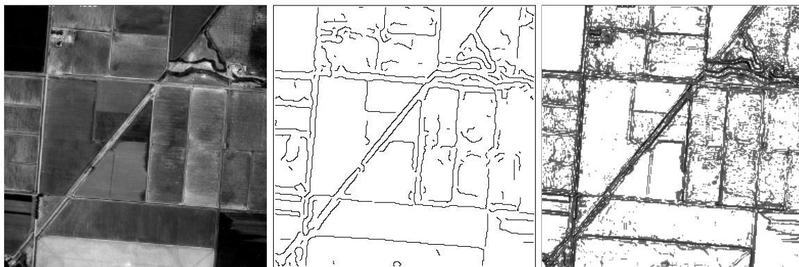
Figure 2. (a) Fields (b) Edges extracted with Canny edge detector (c) Strong Gradient Points Image (edge cover 33%). The gray level of the pixels corresponds to the magnitude of the gradient.
