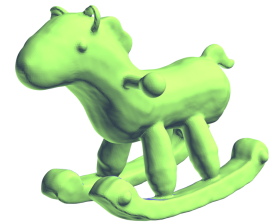
Components: 2; Non-manifold Edges: 0; Non-manifold Vertices: 0; Holes: 0; Genus: 4.
