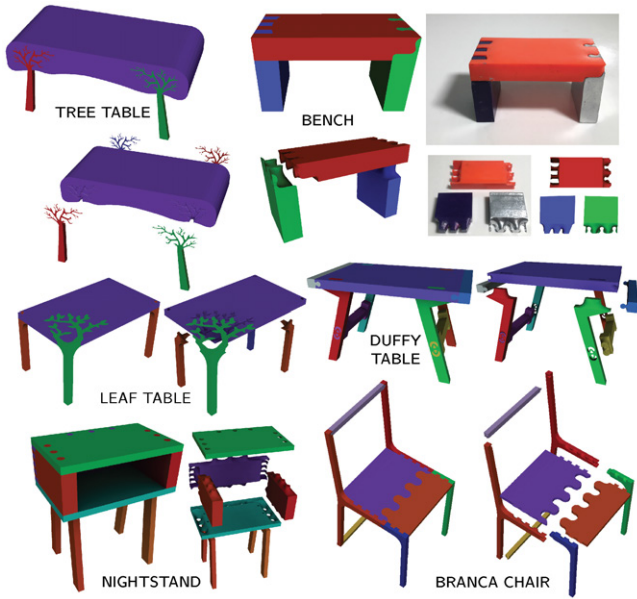
Fig. 15. Partitions of furniture models from Yao et al. [Yao et al. 2017]. Our method found non-obvious directions (validated computationally and via printing) for a few parts, such as the right side of the bench and the side strips on the Duffy table.
