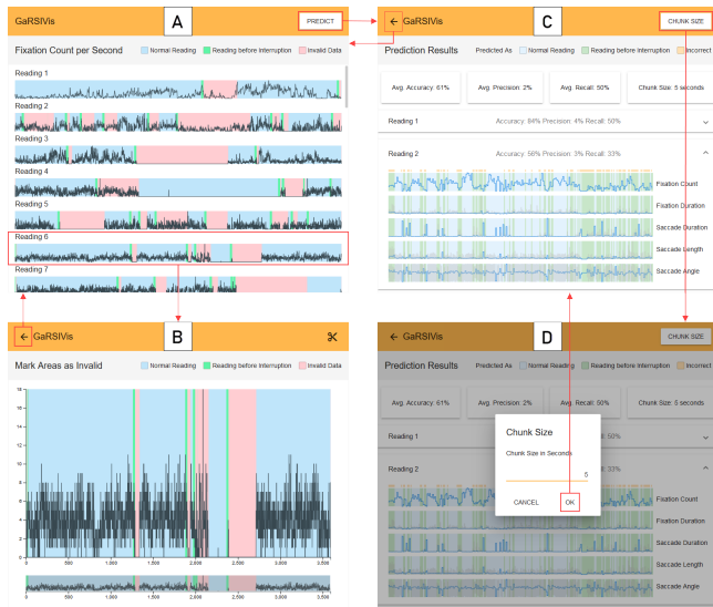
Figure 2: The Overview page (A) with the readings from which analysts can select a particular reading for cleaning. This reading is shown in the Data Cleansing page (B). Upon returning to the Overview page analysts can run a prediction on the cleaned data and view the Prediction Results page (C). From there analysts can choose to rechunk the data (D) and then rerun the prediction on the new chunk size. This workflow can be repeated.
