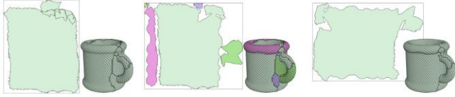
Fig. 14. Overlap removal. After removing overlaps from the input (left), resulting charts (center) can be welded together along a common 3D space seam segment if the parameterization is globally continuous across this segment, and if the combined chart (right) has no self-overlaps. Input has been globally parameterized using [Lipman 2012].
