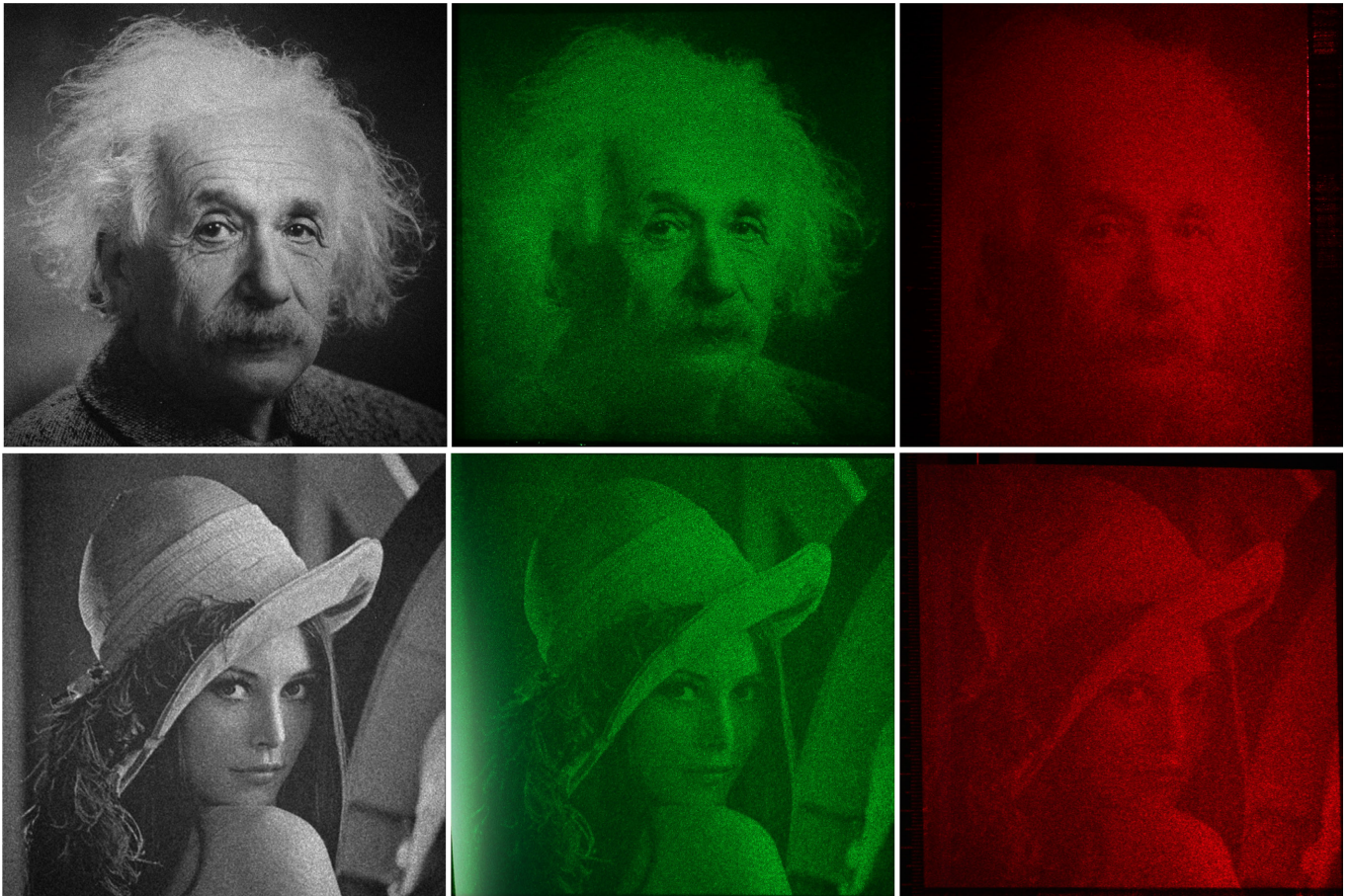
Fig. 8. Comparisons of synthetic (left) images and experimental images (right two) reconstructed from the offset pairing. Notice that all the images have been resampled and integrated over 200\mu\text{m} per pixel subject to human eye's angular resolution at a viewing distance of 50cm. We also note that the intensity distribution of a target image has an impact on the encoding performance, further reflected as the speckle noise level in the decoded image. Specifically, the hair of Einstein exhibits a noisier distribution than that of Lena's hat. Overall, the two decoded gray-scale images are visually recognizable with details preserved. (Albert Einstein Photograph by Orren Jack Turner, Lena image source from Wikipedia)
