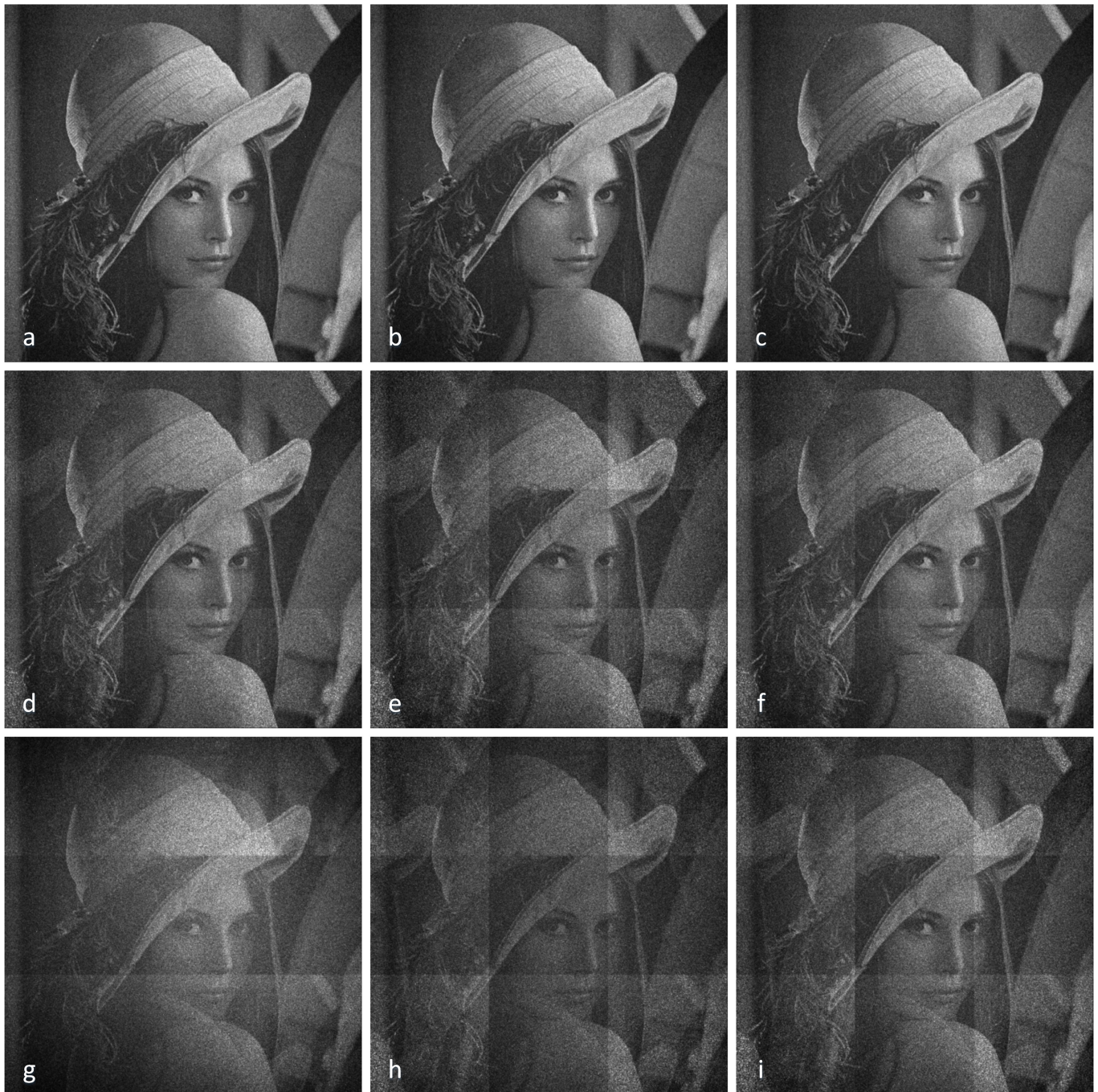
Fig. 7. Comparisons of synthetic images reconstructed from the offset pairing subject to different implementation conditions— (a) perfect condition, (b) weak noise, (c) strong noise, (d) small rotation, (e) large rotation, (f) strong noise + small rotation one (g) directional shift, (h) dual directional shift, (i) strong noise + large rotation, respectively. Notice that all images have been resampled and integrated over 200\mu\text{m} per pixel subject to human eye's angular resolution at a viewing distance of 50cm. (Lena image source from Wikipedia)
