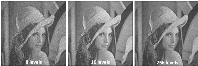
Fig. 2. Comparison of synthetic results with different quantizations. Note that all images are resampled with 8\mu\text{m} on the DOE plane with the final intensity distributions integrated over 200\mu\text{m} on the receiver screen.
