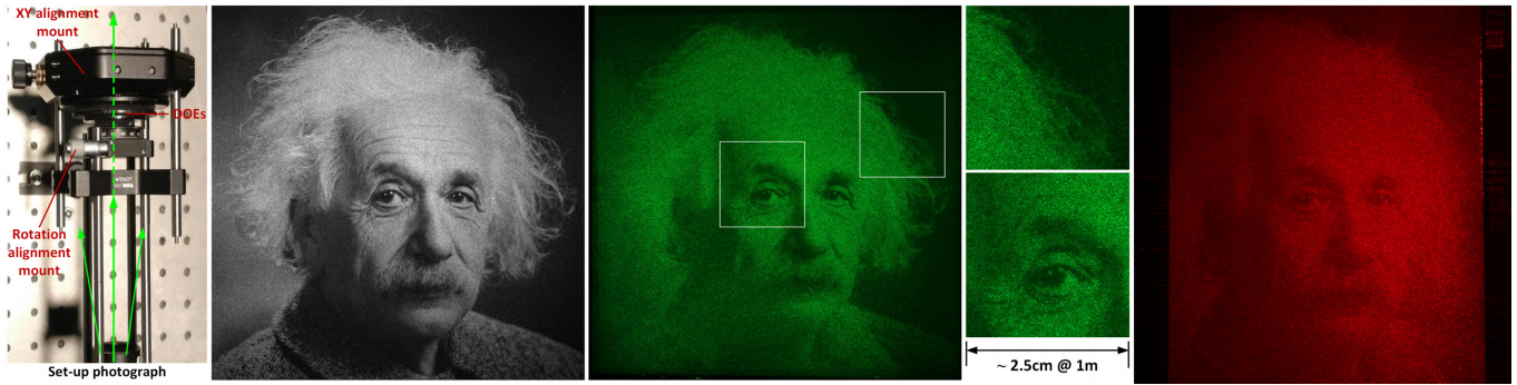
Fig. 6. Synthetic and experimental results of projecting an image through an offset pair of DOEs, with the diagram of set-up indicated (left). We present synthetic results (center left), experimental results illuminated with green laser light (center right), and experimental results illuminated with red laser light (right-most). The size of DOEs are 1.4cm by 1.4cm individually, and the projection distance is set 1m. The final projected image size is around 12cm by 12cm. (Albert Einstein Photograph by Orren Jack Turner)
