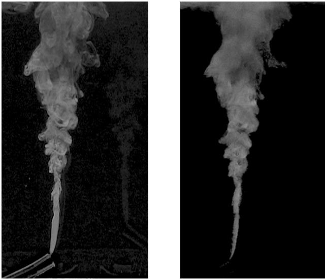
Figure 7: 95% isopropyl alcohol and fluorescein-sodium rising under buoyancy after injection into standing tap-water. Camera view (left) and grid-free stochastic tomography reconstruction (right) from 15 views re-rendered from a similar viewpoint. Many fine scale features of the transition from laminar-flow to turbulent-mixing are captured by the rendering, however minor camera misalignment limits the reconstruction resolution. Please see the supplemental material for the corresponding animated sequence. This reconstruction used 200 million mutations and 10 thousand sample chains with no regularization. Computation time: 14 min/frame.
