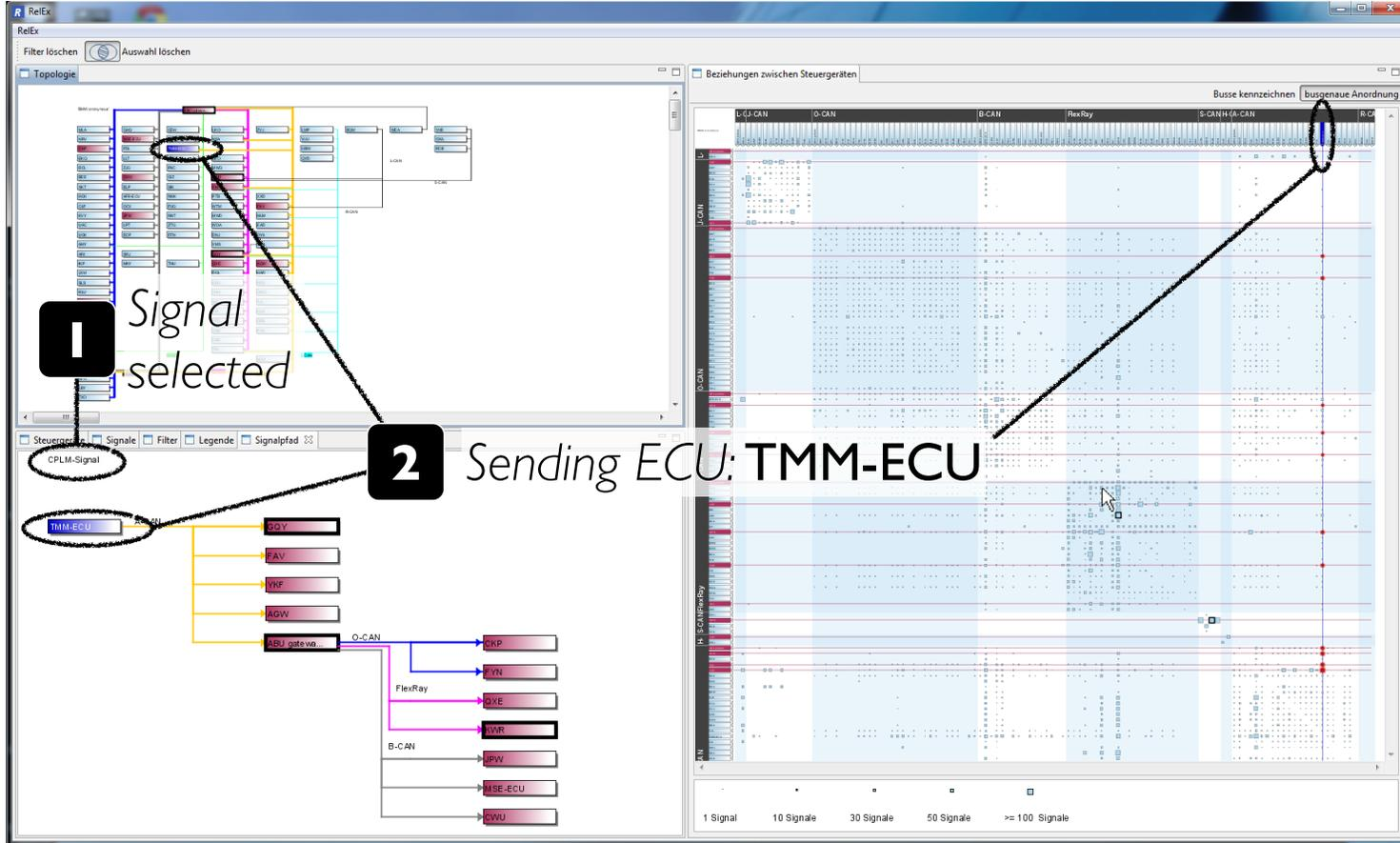
Figure S5: Example 2: Inter-bus communication. The user selected the CPLM-Signal (1). The sender of this signal is the TMM-ECU (2); it is highlighted in blue in the Topology View (upper left), the Matrix View (right), and the SignalPath View (lower left).
