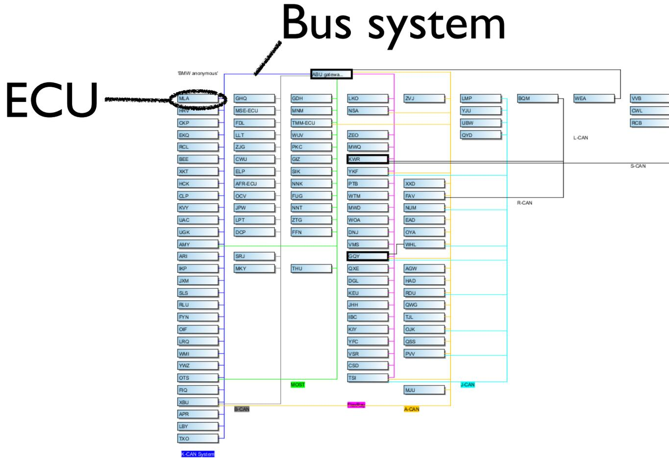
Figure S1: Topology View: The basic visual encodings are the rectangles for *ECUs*, and color-coded lines for *bus systems*.
