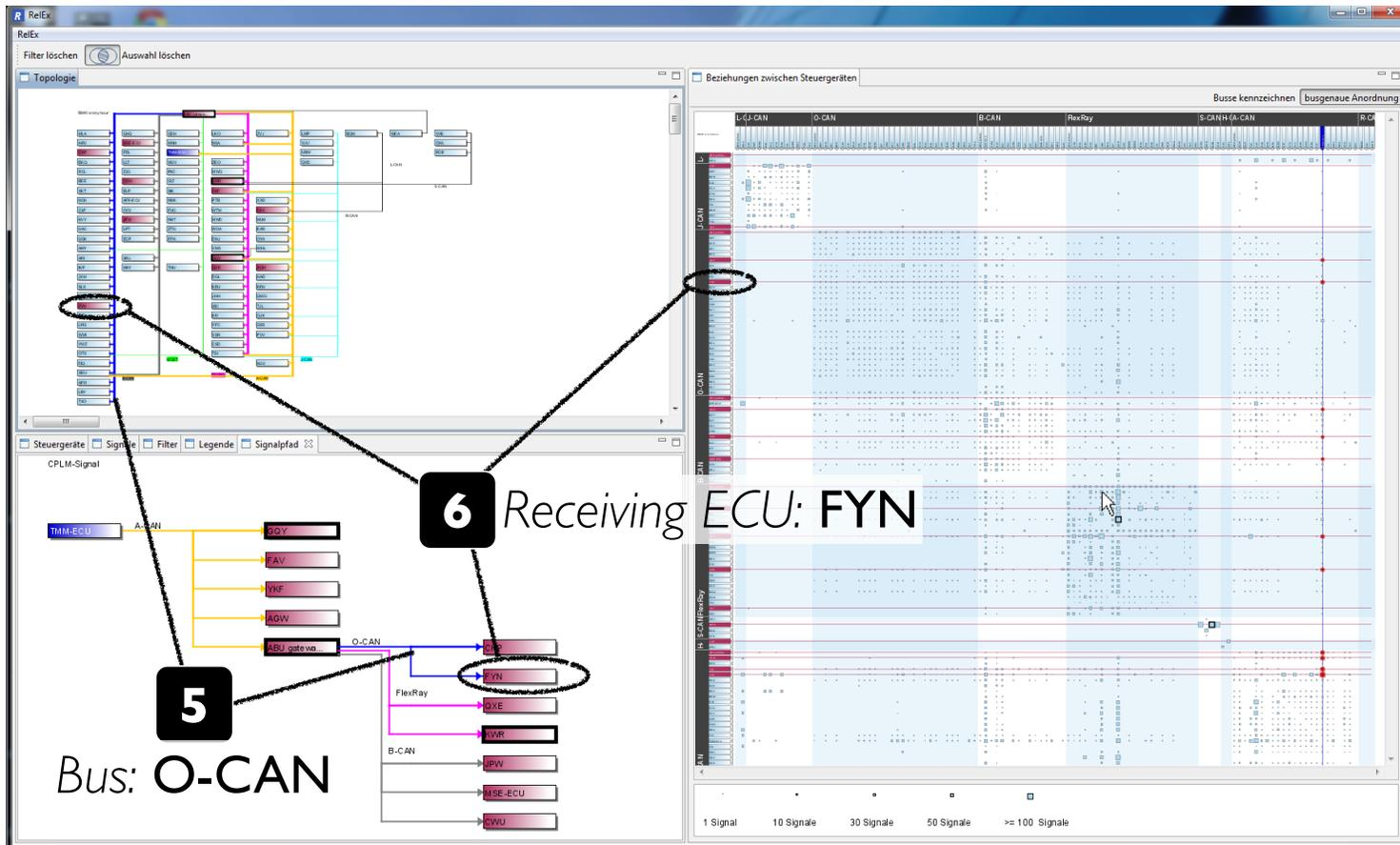
Figure S7: Example 2, continued. One of the bus systems also connected to the ABU gateway is the blue O-CAN (5), transferring the signal to two receiving ECUs: CKP and FYN (6). The communication between the sender TMM-ECU and the receiver ECU FYN is thus an example of inter-bus communication.
