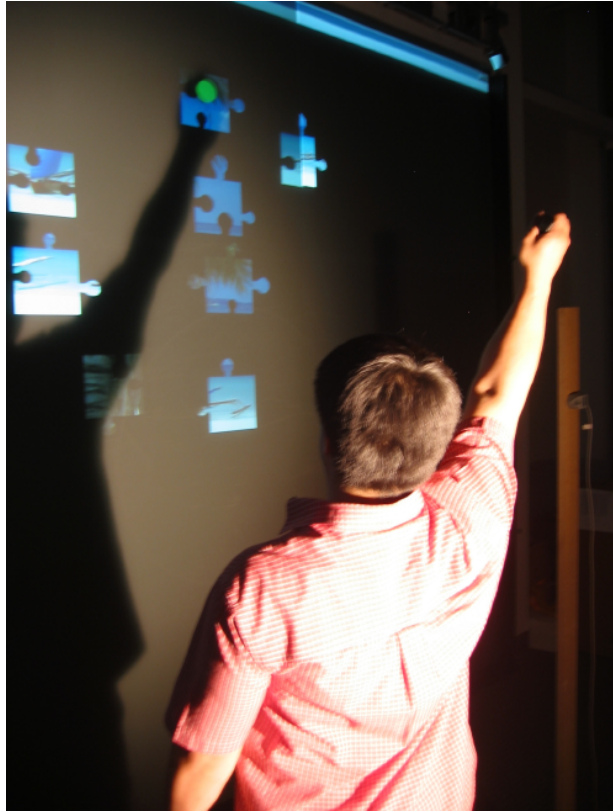
Figure 3.5: Shadow Reaching prototype 1. A physical shadow is cast with a bright lamp. The user's hand locations are measured using trackers. Cursors are rendered on the display near the shadow.
