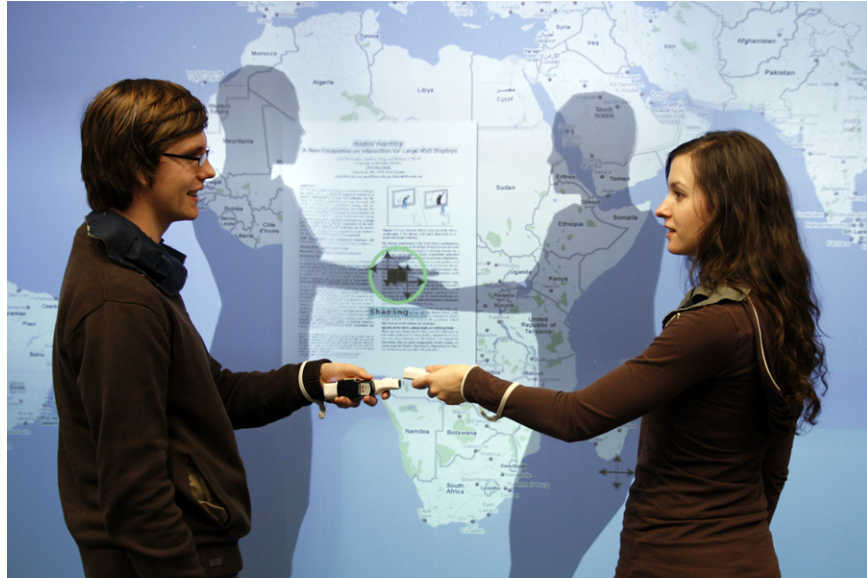
Figure 4.8: A user passes a private document to a collaborator. The sharing protocol requires close physical proximity, and encourages direct eye contact. Feedback on the screen is a green circle surrounding the projection of the two users hands, to indicate a successful pass.
