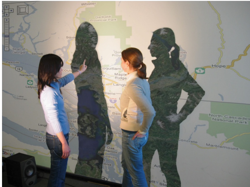
Figure 3.9: A mockup of users interacting using Magic Shadows. Their shadows display satellite photos, while the context display maps.
