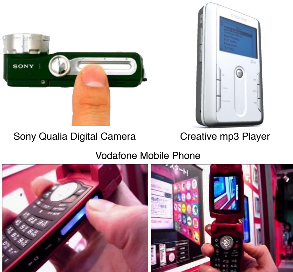
Figure 3.2: Examples of existing products utilizing linear capacitive touch sensors.
