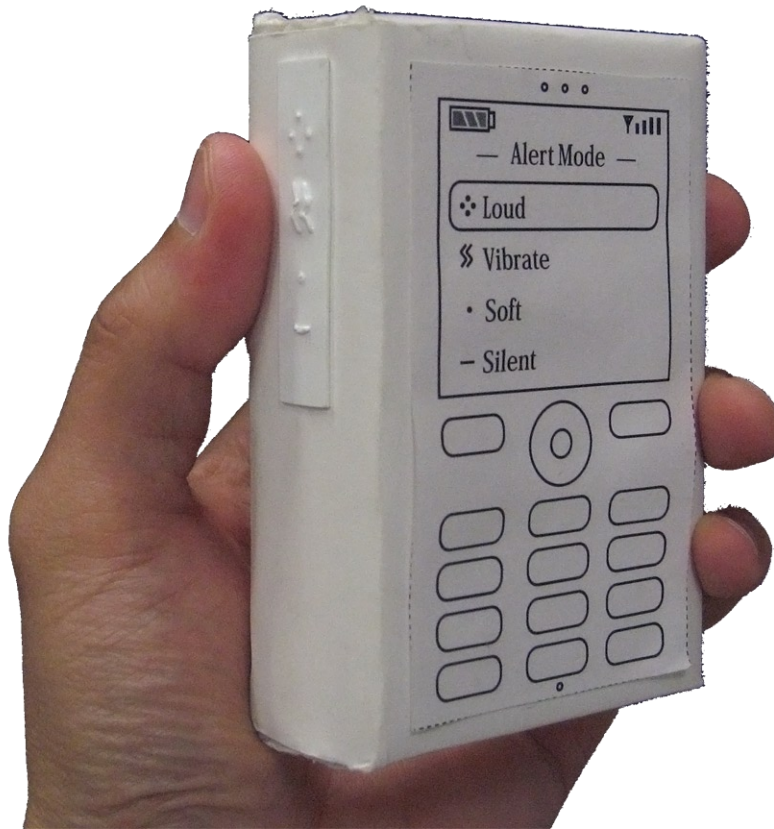
Figure 3.7: Low-fidelity foam mockup used for early user evaluation of the menu selection application concept. There is a textured plastic tactile strip mounted on the left side of the mockup.
