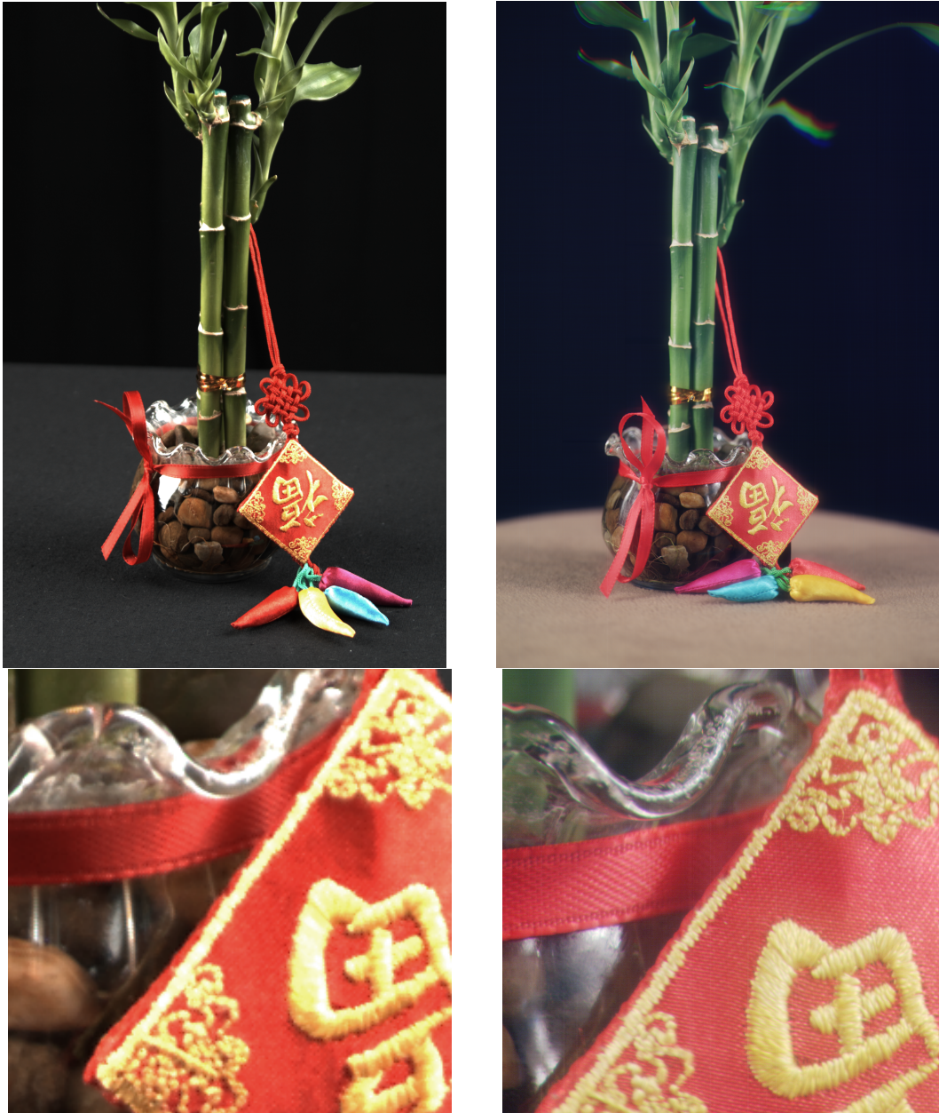
Figure 5.2: Comparison between the Canon EOS D60 (left) and our scan camera (right). The top row shows slightly cropped images. The bottom row shows magnification of one region to better compare the resolution.
