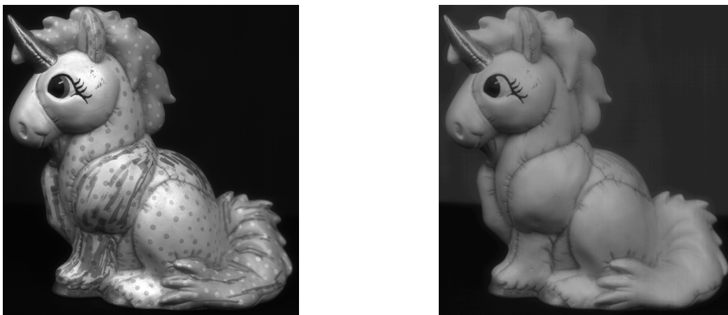
Figure 4.4: Comparison of a grayscale photograph (left) with an infrared photograph (right). Note that except for the black color of the eye, the effect of different paints is almost completely removed in the infrared image.
