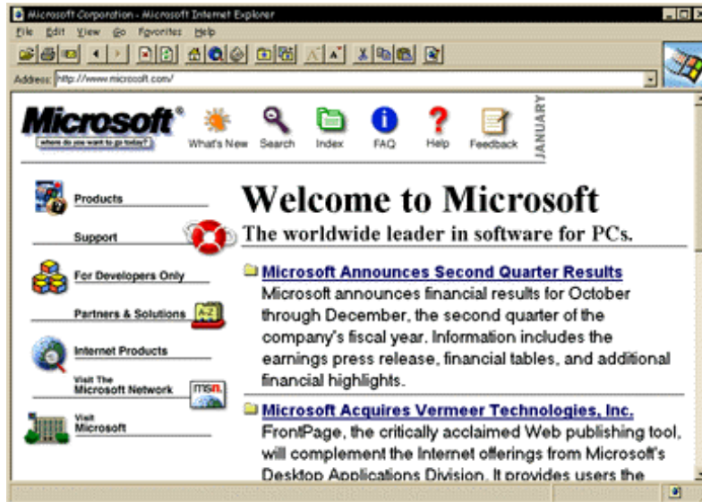
Figure 4: Microsoft Internet Explorer WWW browser showing inline images, formatted text, and hyperlinks embedded in the HTML page
