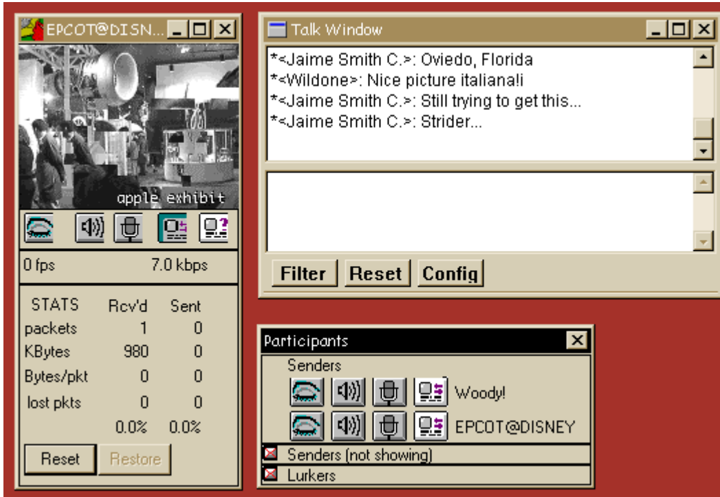
Figure 3: CU-SeeMe conferencing application which renders compressed video and audio streams and out-of-band text “chat” messages.
