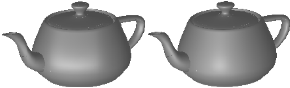
Figure 5.6: Two teapots rendered with an anisotropic BRDF representing brushed metal and the transformed isotropic version
