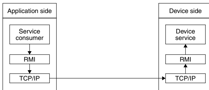
Figure 14.6. Device service with RMI support.
