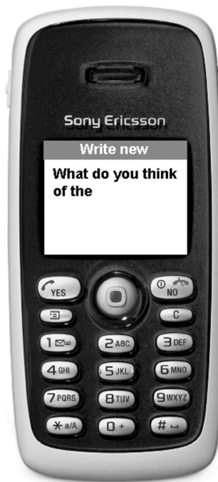
Figure 15.5. A typical device that benefits from Tegic T9, the Sony Ericsson T300 mobile phone. Characters are entered by using pushing once on the keys 2–9, while key 1 is used for spacing between words.
