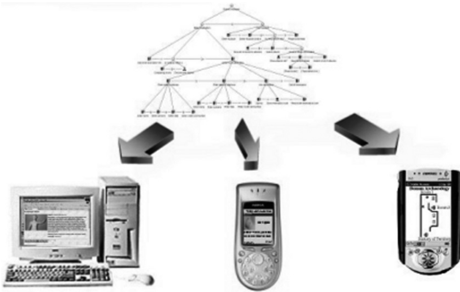
Figure 11.6. Deriving multiple user interfaces from a single task model.
