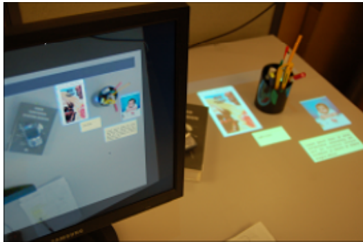
Fig. 1. The DeskJockey System where digital information can be placed on a physical desk, amongst other physical artifacts that reside in this space
