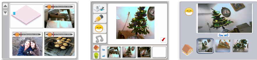
Fig. 4. The final concept has an initial screen to retrieve stories or to start creating a new story ( left ), while creating or editing storyline clips is done by means of an interface that offers four input modalities: pictures, annotation, emotions, and sounds ( middle ). Finally an interface is made for showing and browsing the story created by a user ( right ).
