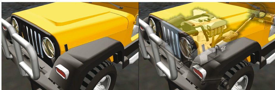
Fig. 1. Dynamic transparency uncovering an engine inside a jeep
