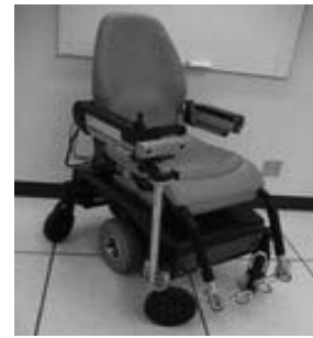
Figure 1: NOAH wheelchair system prototype (a commercially available powered wheelchair equipped with a stereovision camera and a laptop placed under the seat).
