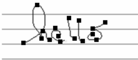
Figure 4. Ink strokes are segmented at local Y extremes and placed into an ink word.
