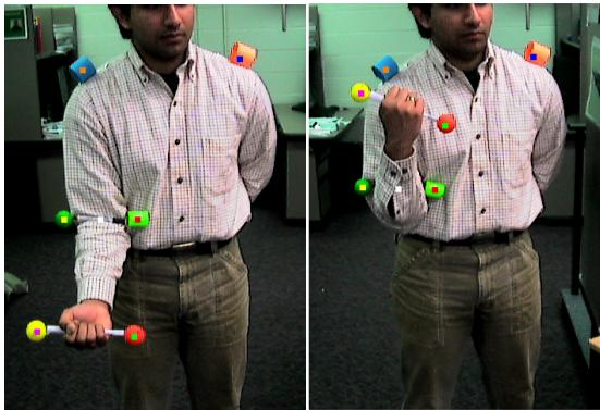
Figure 1: Shows the position of the tracked color markers to detect user's torso and arm exercise posture.
