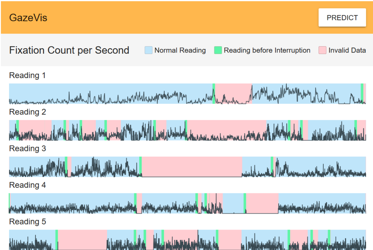
Fig. 1. Overview of GazeVis interface showing a list of readings along with their associated fixation counts. The colors indicate regions that correspond to normal reading, reading before self interruption, and invalid data.
