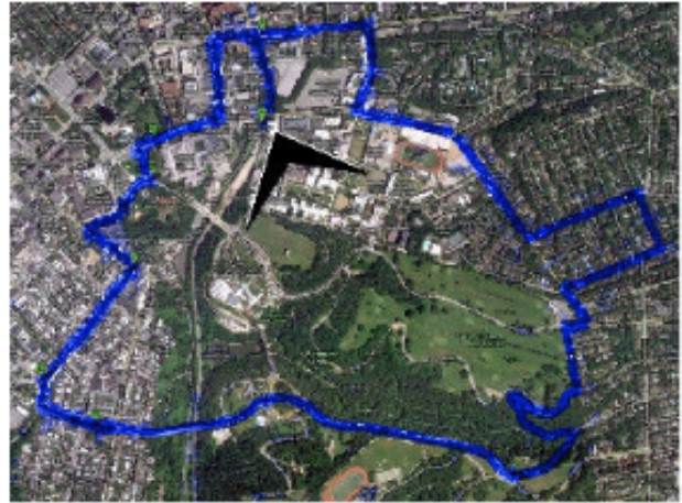
Figure 6. The camera trajectory in an 8 km route. The height of the camera is assumed constant and the orientation of the camera is fixed (looking forward on the road). The reference is from Google map. Figure from [1].
