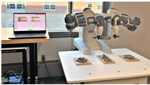
Figure 4: Experimental setup: Participants used a touch-screen-enabled laptop (left) to program a two-armed collaborative robot (right).
