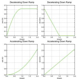
Figure 4: Theoretical and our numerical results for two tests of a block sliding down an inclined plane with friction. The curves lie on top of each other in the figures due to the accuracy of our new time sequencing algorithm.
